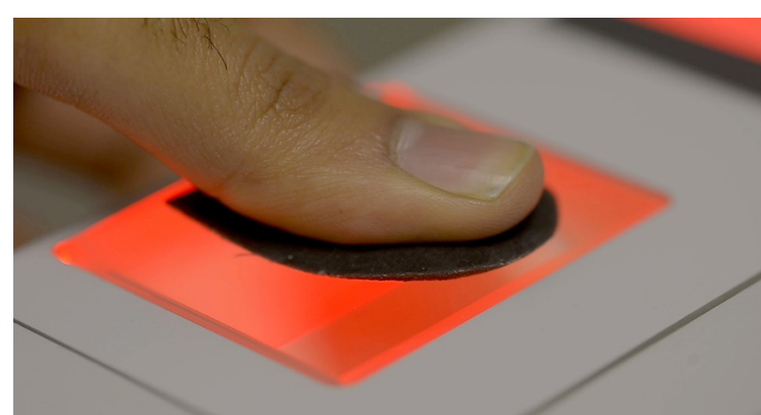
Figure 2: 3D Printed Fingerprint Used on a Scanning Device (Image by Michigan State University)
